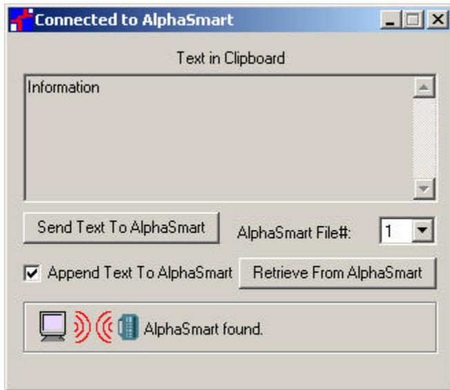
3. Align the AlphaSmart's infrared port lens with the lens of the computer's IR Pod or built-in IR device and press the Send button. (Even though you are not sending text from the AlphaSmart, this step is necessary to open the IR connection.) The AlphaSmart will display messages indicating that it is connecting to the PC. After a few seconds, the Get Utility will show that an AlphaSmart has been found.
